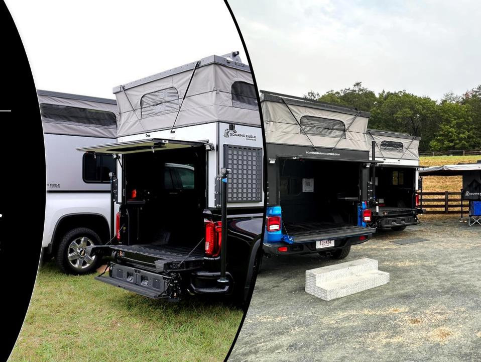
Some of our competition cut the corners out of their rear door which limits the size of things you can load into the back of the truck.
