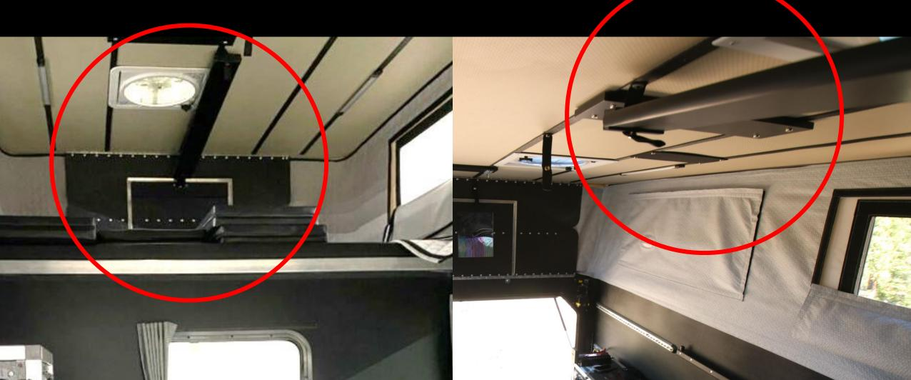
Some manufacturer's use thin, composite board pieces that swings up to support the weight of the very thin roof.
