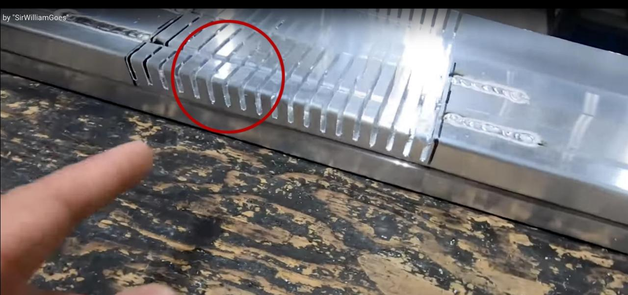
Is there Weight Savings by doing this? Sure – but at what Cost? The answer to that is Structural Integrity, which is completely lost.
