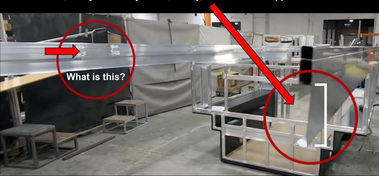
This is how they form their Radius "Structure" - by Notching their Thin Aluminum Tube <u>and</u> C-Channel every 1/4" so they can bend it.
